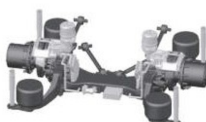
E-driven axle BRE 131 (Developing phase)
