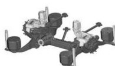
Low floor bus driven axle BRA 132DC80/83/90
