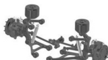
Low entrance and low floor bus front axle BFA 80I
