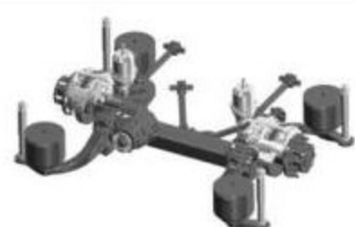
Low floor bus driven axle BRA 101DC80/90
