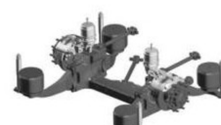
Low floor bus non-driven portal axle BDA 132
